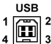
Figure 3-4: USB Connector pin orientation.
